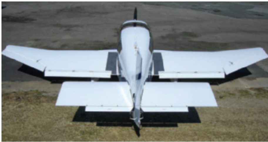
Above: cranked wing and large all-flying tailplane make for a sweet-handling, stable aircraft
