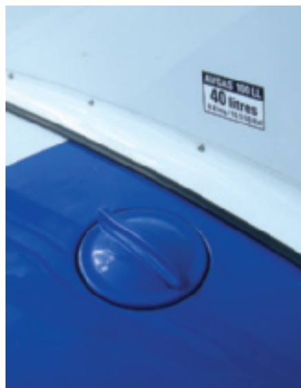
Below right: wing tanks each hold 40 litres, comfortably enough for an hour; main tank holds 110 litres
