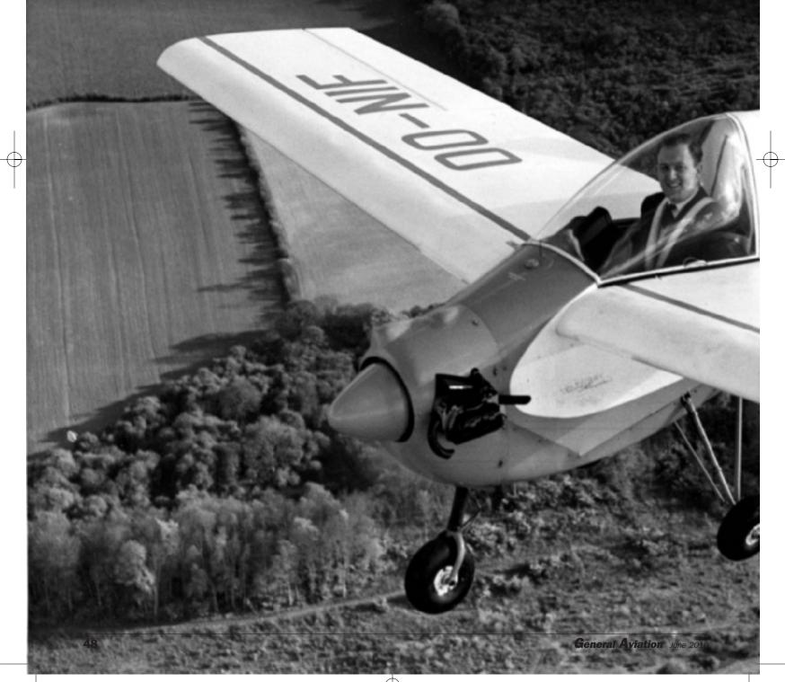
Among the Nipper's many favourable features is a good view in most directions (with downward vision panels in the wing roots) an all-flying fin/rudder, a simple undercarriage with disc brakes and an ingenious facility for accommodating a large person in a very small cockpit. The prototype took to the air late in 1957 and all early specimens were Belgian built, appearing on the market about 18 months later at a flyaway at £818.
