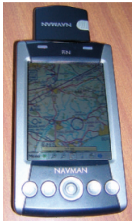
Above: early PDA/GPS kit – Compaq PDA with RS232 connection and NMEA data from an Etrex Right: Navman PIN has GPS receiver built in, but needs bulky power connector
