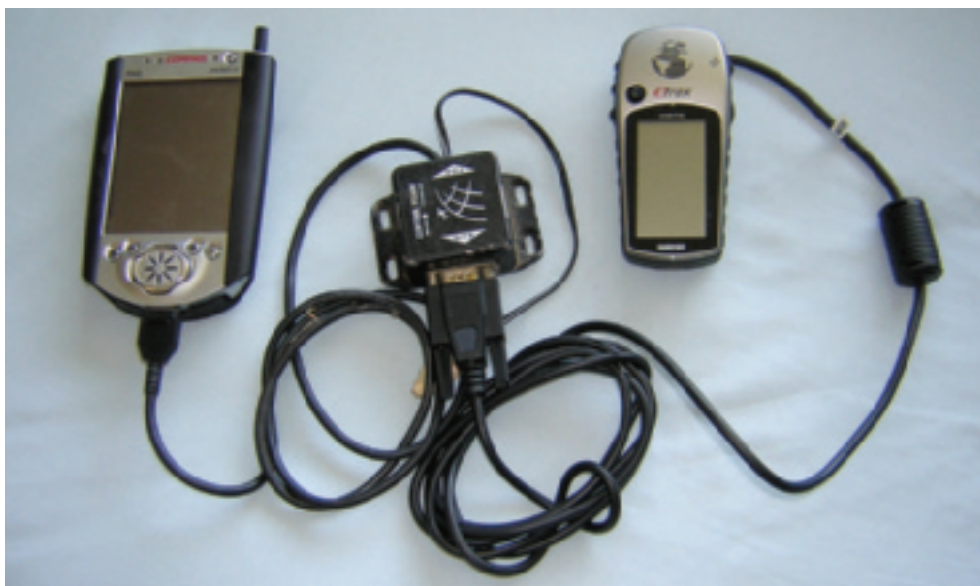
Above: early PDA/GPS kit – Compaq PDA with RS232 connection and NMEA data from an Etrex Right: Navman PIN has GPS receiver built in, but needs bulky power connector
