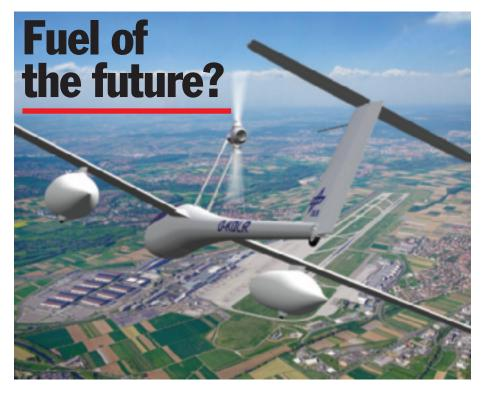
Is this the answer to our avgas problems? Chemical company BASF and the DLR Institute of Thermal Dynamics in Stuttgart have designed the first manned aircraft that can take off and fly solely on the power of a fuel cell.
