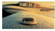
often underestimated. It commonly accumulates on aircraft overnight, particularly when the sky is clear, and forms because the aircraft's body becomes cooler than the outside air. This process is known as radiant cooling, and while only a few degrees difference is needed, it's not uncommon for the aircraft skin to actually be as much as 5°C or, in very severe conditions, 10°C cooler than the outside air temperature.
