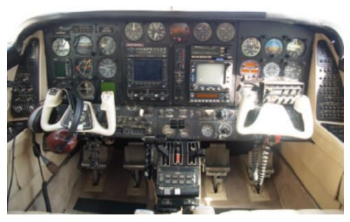
Left: de-icing panel includes fuel vents and dual pitot heaters as well as windshield, boots and electric prop heater
