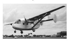
Above: G-AHDM was fitted experimentally with a very high aspect ratio wing of 75ft span designed by Hurel-Dubois of Villacoublay in France
