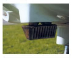
Left: quiet prop on a Swedish Cherokee - the cost of UK regulation prevents it Above: Liese silencer on the same aircraft gives a 7db noise reduction Right: where will tomorrow's maintenance engineers come from?
