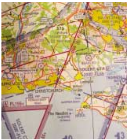
You could bust the Solent 2,000-foot Class D Zone on the tip of the Isle of Wight
