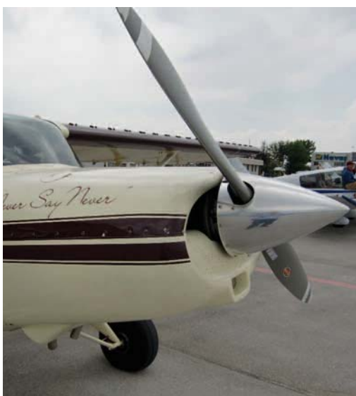
Left, top to bottom: vortex generators on the wing improve control at low speeds Two-thirds span flaps can be set to minus seven degrees Big tyres are essential for African bush strips Harzell constant-speed prop gets the most out of the Lycoming 180
