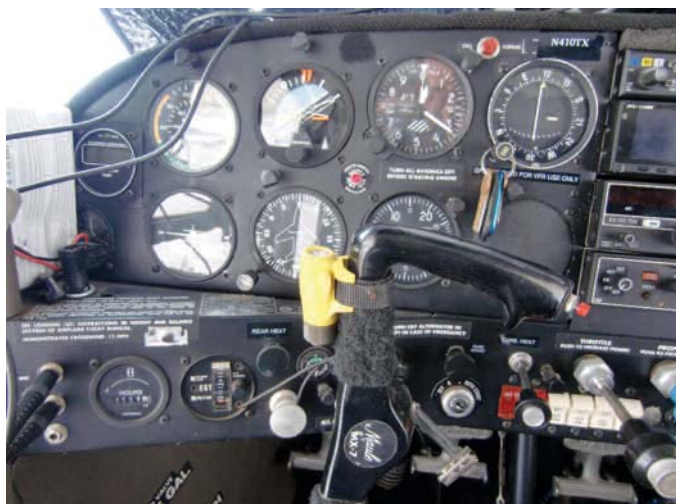
Right: bush-plane spartan, the Maule's front office is utilitarian rather than plush Below: left-seater faces a basic-T panel and little else, but it's enough Below right: the fuel transfer controls and Ts and Ps fall to the right-seater
