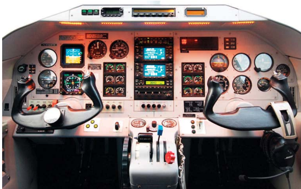
Lower left: electrical switches and circuit breakers fall easily to the pilot's left hand Below: by the standards of complex singles, a clean and uncluttered panel Bottom: centre console has cabin pressurisation dial and readout on top
