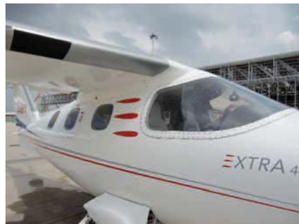
Far left: serious amounts of legroom improve passenger comfort on long trips Left: pressurisation system means windows are smaller than in other GA aircraft Lower left: clamshell doors incorporate a step in the bottom half
